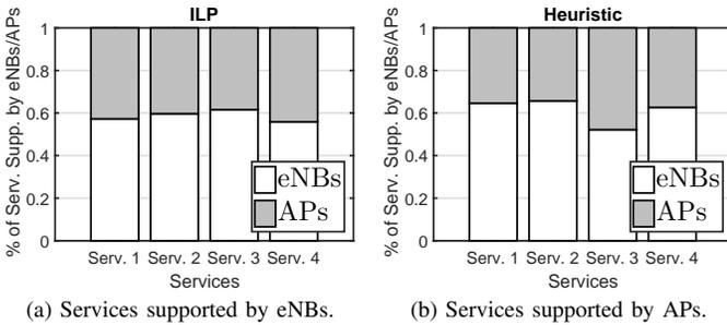
Fig. 2: Distribution of the 4 possible service classes across both eNBs and APs using the different user association algorithms.
