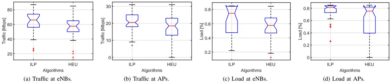
Fig. 1: Traffic and load distributions at eNBs and APs after 150 association requests for all algorithms.
